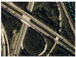
Figure 5. Clipping from a film animation showing moving vehicles on a freeway interchange north of Munich, blue=slow vehicles, orange=fast vehicles
